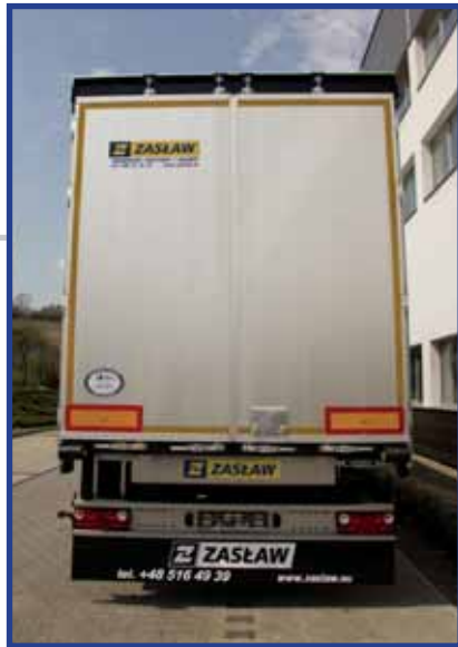
Reinforced rear door made of aluminium panels
