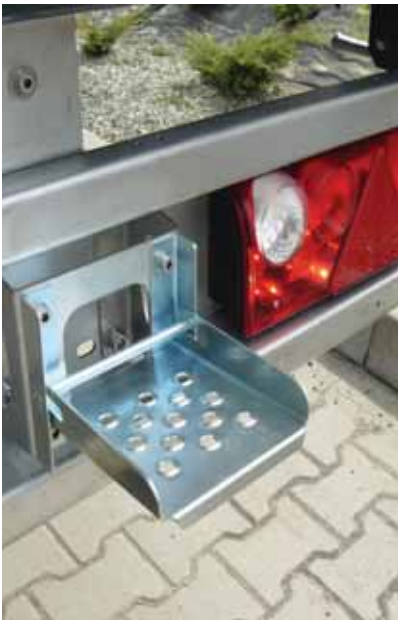
Rear bumper made of stainless steel with a step facilitating entry on the trailer
