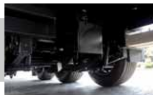
Central lifting of the first axle
