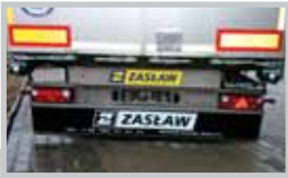
Rear bumper made of stainless steel
