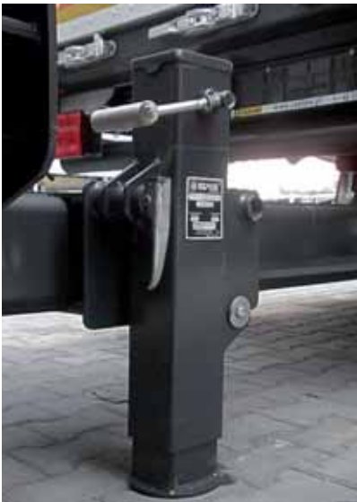
Telescopic landing leg, optionally mechanical landing leg – 1 leg mounted on the drawbar and 2 legs mounted in the rear part of the trailer for stabilization of the unhitched vehicle
