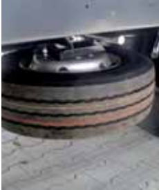
Truck spare wheel carrier, spare wheel with carrier for the trailer
