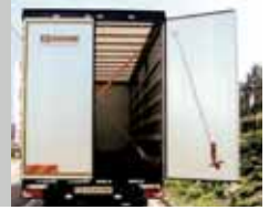
Aluminium rear door up to the roof level with internal bolts and pole for roof handling
