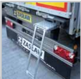
Entry ladder – steel, galvanized
