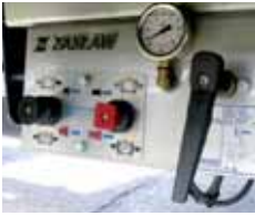
Parking brake console, H-S platform levelling valve, manometer
