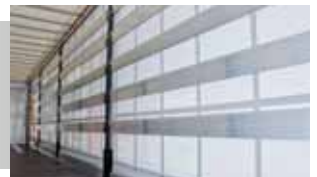
Construction of upperstructure reinforcements depending on EN 12642 XL certificate
