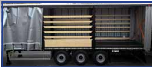
Possibility of stacking planks to use them as side board
