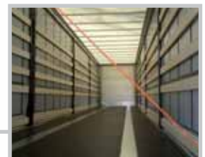
Floor made of 27 mm thick anti-slip plywood, screwed and sealed
