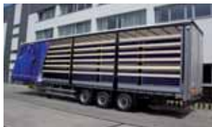
Upperstructure with roof liftable for loading and with two internal heights for driving
