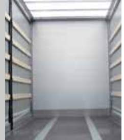
Front wall made of aluminium profiles, sliding side pillars, side wooden planks (possibility of choice of aluminium planks), floor made of 27 mm water-resistant anti-slip plywood
