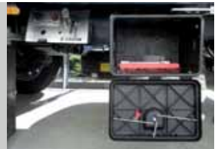
Console of pneumatics control and axle load manometer, plastic toolbox with equipment
